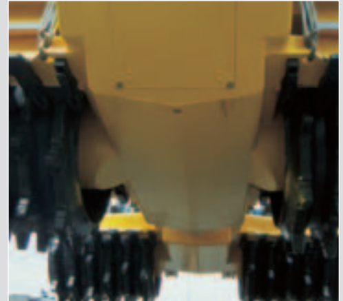
The sealed tub design protects all drive components
