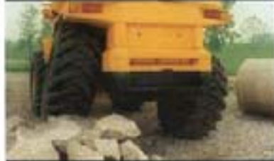
Rear axle oscillates 22 degrees for firm footing on rough terrain.
