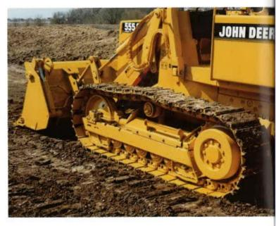
Large boron steel track rollers are hardened through the wear limit inside and out for long life. Irregular spacing causes bottom rollers to contact links at varying points for a smoother, quieter ride.
