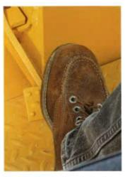
Decelerator is standard with either transmission. Fully depressing the pedal declutches the transmission, slowing ground speed to a virtual crawl. Use it for close-up work around footings or when loading trucks.
