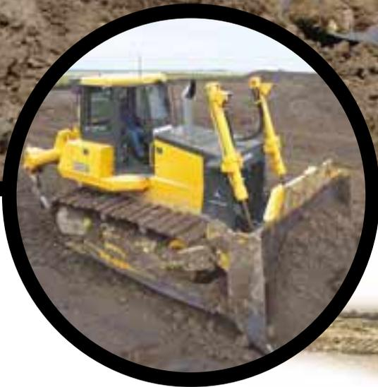
Infinitely variable track control lets you speed-up or slow power to each track – for smooth, full-power turns that don't tear-up soft terrain like clutch/brake systems.
