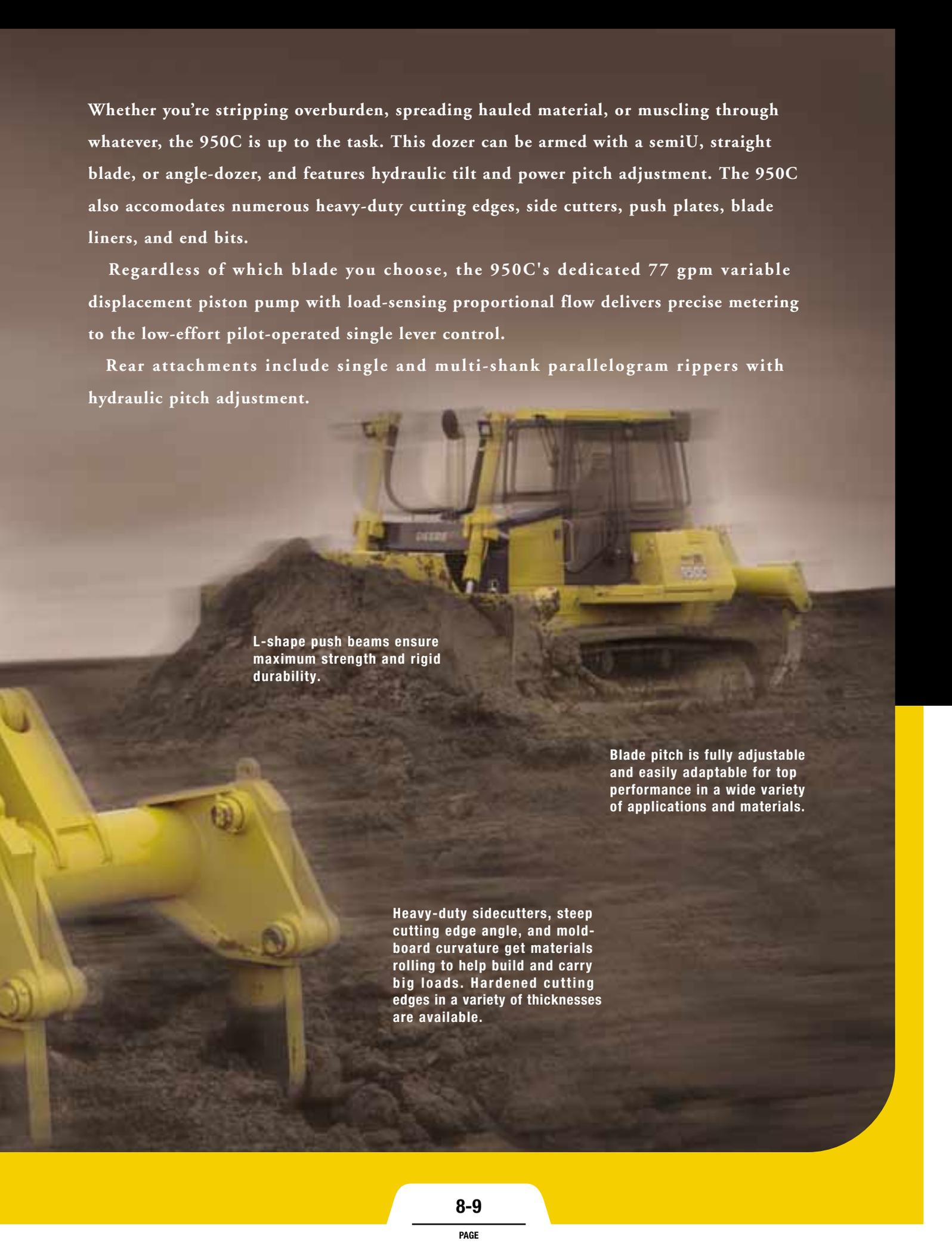
L-shape push beams ensure maximum strength and rigid durability.
