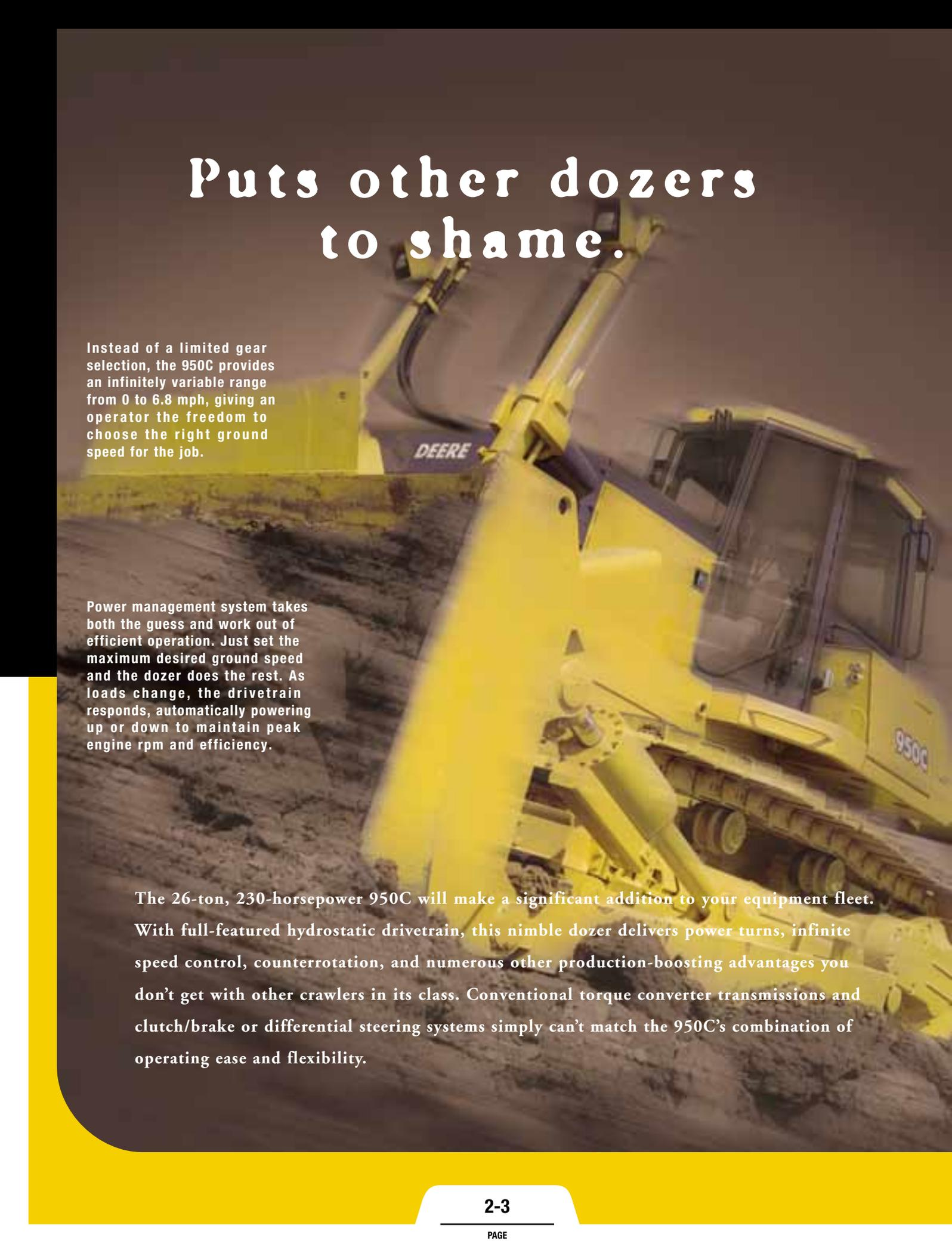
Instead of a limited gear selection, the 950C provides an infinitely variable range from 0 to 6.8 mph, giving an operator the freedom to choose the right ground speed for the job.
