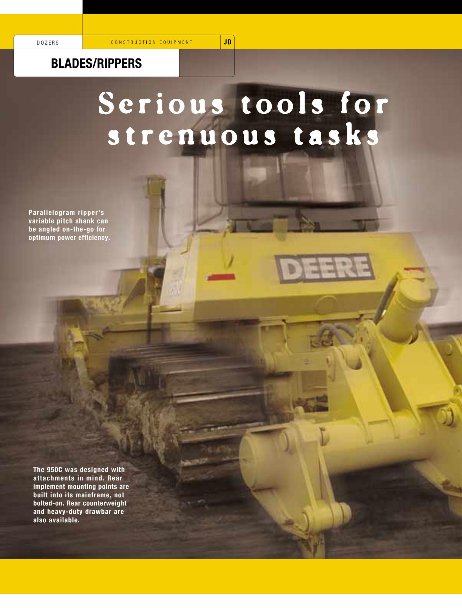
Whether you're stripping overburden, spreading hauled material, or muscling through whatever, the 950C is up to the task. This dozer can be armed with a semiU, straight blade, or angle-dozer, and features hydraulic tilt and power pitch adjustment. The 950C also accomodates numerous heavy-duty cutting edges, side cutters, push plates, blade liners, and end bits.
