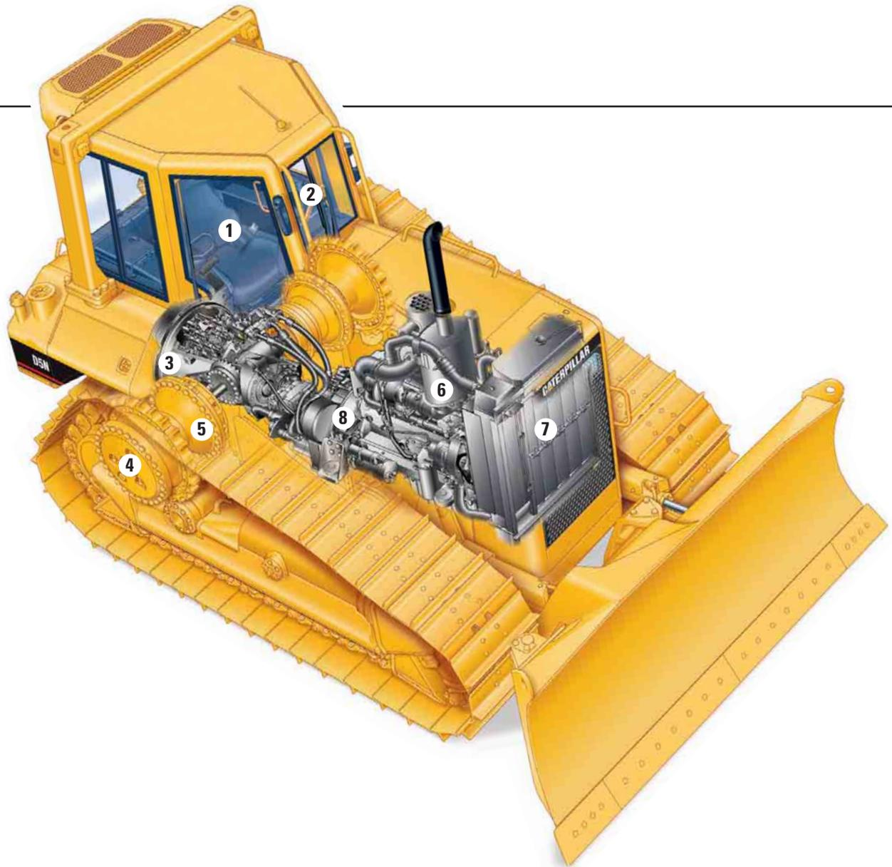
**1 Operator's Station.** State of the art operator's station has reduced sound levels, lower cab vibration, and increased glass area.
