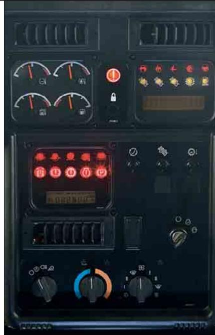
**Dash.** The instrument panel, with easy to read analog gauges and warning lamps, keeps the operator aware of any potential problems. All gauges and readouts are easily visible in direct sunlight. HVAC controls and vents are conveniently located on the dash to provide climate control for the operator. Auto-shift and Auto-kickdown controls are located within easy reach of the operator. New footpads keep the operator stable and comfortable during side slope applications.
