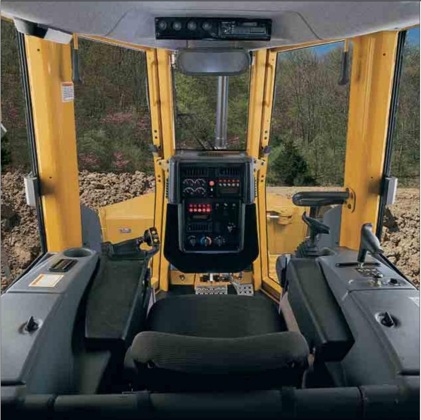
**Cab.** The cab incorporates large glass window and door panels. This allows for excellent visibility to the blade, rear and sides of the machine. New door and window seal design allows for a fully pressurized dust free cab. Low acoustic headliner material, and sound suppression foam panels reduce sound levels to below 75 dB(A) when measured per ISO 6394:1998.
