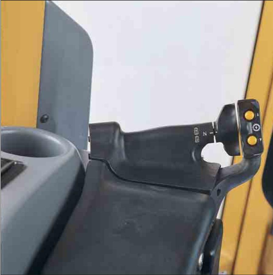
**Three Speed Forward/Reverse Gear Selection.** Three speed forward/reverse gear selection is achieved simply by pressing the yellow speed selection buttons. These buttons are integrated into the Finger Tip Control group.
