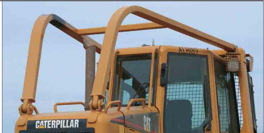
**Forestry Sweeps.** In forestry and land clearing applications where limbs and debris can damage a machine, optional sweeps are available for the N-Series. Sweeps help to shield critical components on the tractor such as hydraulic lines, exhaust stacks, cab windows and lights from damage.
