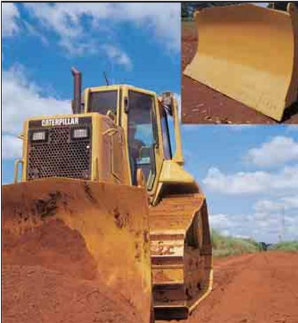
**Caterpillar Blades.** With superior moldboard and 4-cell structure design, Cat bulldozer blades hold up to the toughest job conditions. Our high-tensile strength blades resist torsional bending and deflection in tough applications.
