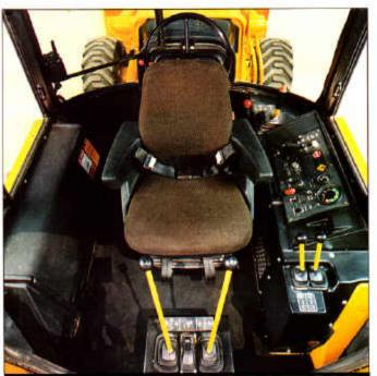
The industry standard. Large door swings open to the front, can be left open during operation. Sixtysix percent of the glass area opens for superior ventilation. Electronic monitor provides audible and visible warnings for vital functions. There are four seat options and three control options.
