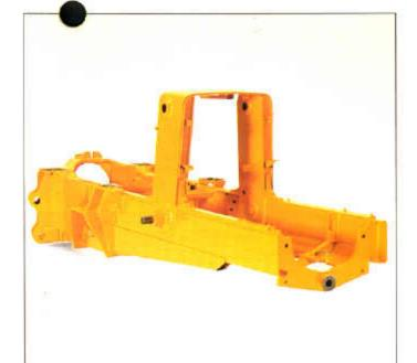
All drivetrain components are mounted independently to the massive unitized mainframe where they are isolated from working stress and shock loads. And each drivetrain component can be removed independently of the others to speed repairs, reduce downtime.
