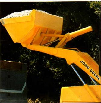
A single dump cylinder on the loader bucket gives the operator an unobstructed view to the bucket. Simpler linkage and one less cylinder reduces weight. It also means there are fewer pivot points and fewer lubrication points reducing maintenance time and expense.
