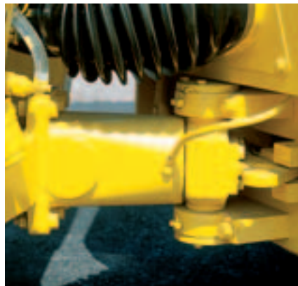
Bolt-on oscillating, articulation joint for long life and easy replacement or repairs (BW120AC-3 Shown)
