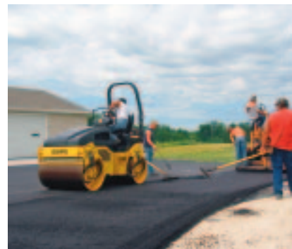
BW120AD-4 shown with optional folding ROPS.
