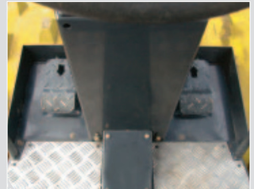
Optional blade system(s) is controlled by strategically positioned floor mounted foot pedals..
