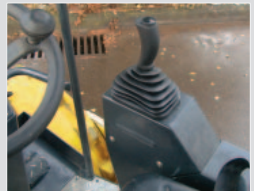
Right hand console positioned travel control lever easily regulates travel direction and speed.
