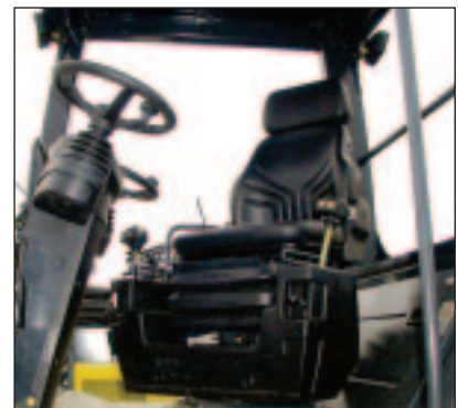
BW 141AD-4 / BW 151AD-4 Operator's platform with sliding/swiveling seating position
