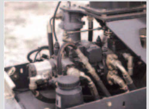
Dual travel pump design of the DH / PDH-3 models further enhances tractive effort and gradeability.
