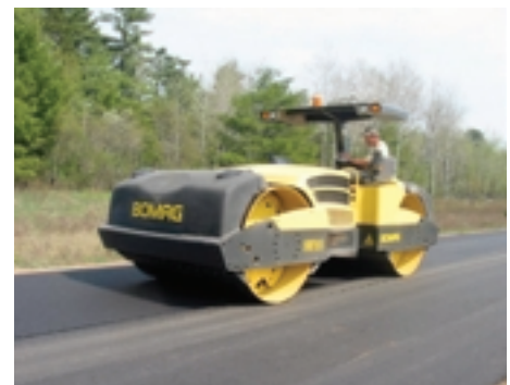
84" rolling width with available 4000 vpm frequency.
