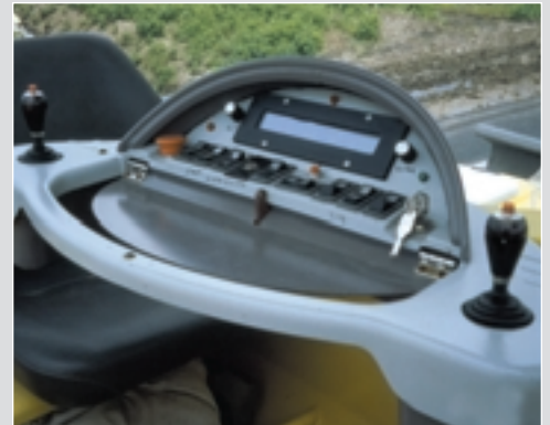
Operator's control panel is fully adjustable to either seating position. Simplified controls make operation easy to novice, as well as experienced operators. Display panel provides all necessary, as well as critical information for proper machine operation and professional results.
