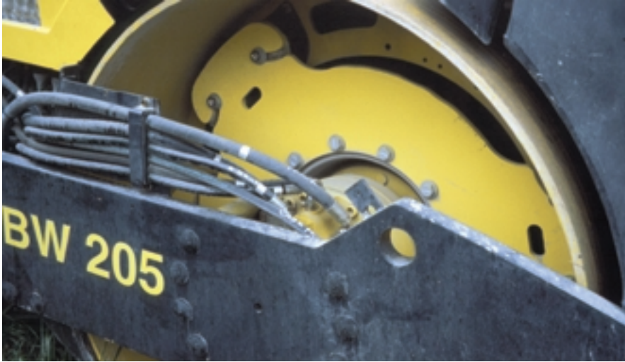
Direct drum drive with vibrating travel speeds of 4.5 mph available. Individually serviceable isolators without drum removal.
