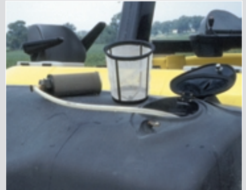
Waterspray system is further protected by fill port strainer and in-tank suction filtration. Fill port cover is lockable for vandal protection.
