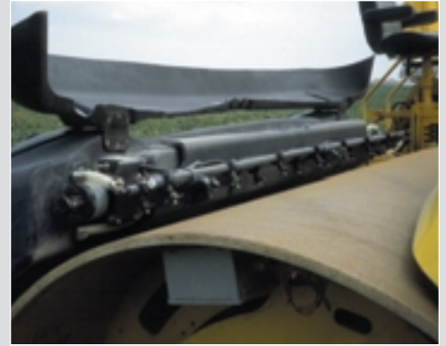
Dual, independent spray systems per drum, with quick-disconnect nozzles, ensure continuous waterspray operation. Spray pattern protected by hinged, swing-up wind deflection covers.
