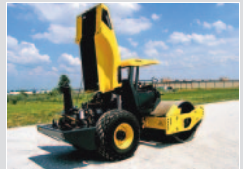
Vertically Opening Hood for Maximum Serviceability
