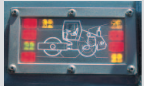
Audible and visual warning indicators on the platform's diagnostic panel alerts the operator of potential service problems
