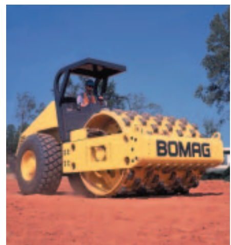
Designed specifically for soil compaction.
