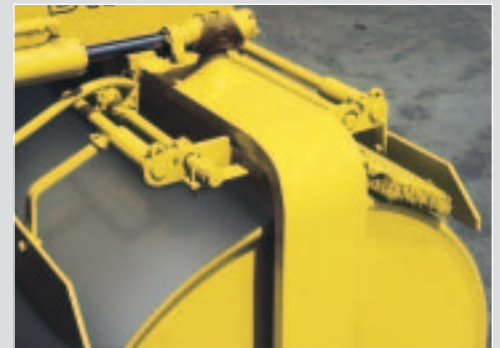
Each drum has a full width cocoa mat, two scraper bars that clean in both travel directions, and four spray nozzles
