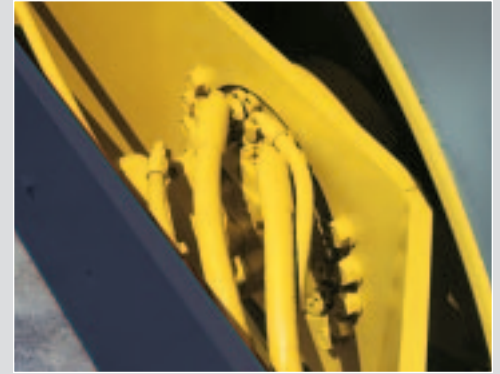
The full hydrostatic drive with a low-speed, high-torque motor delivers smooth acceleration, deceleration and directional changes.
