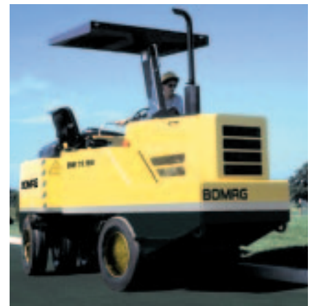
BW11RH in action on an asphalt resurfacing application
