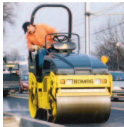
BW100AD-4 rolling a curbline.
