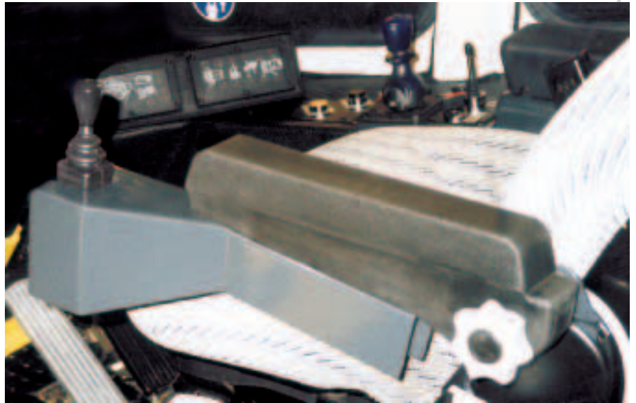
Ergonomic control layout including joystick steering control.
