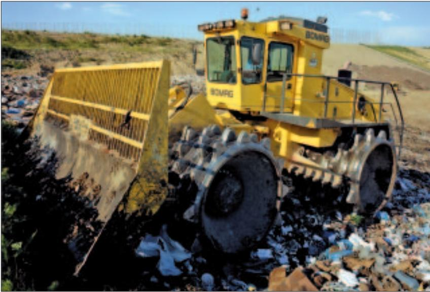
More efficient utilization of available engine horsepower through the BC972/1172RB-2's hydrostatic drive system
