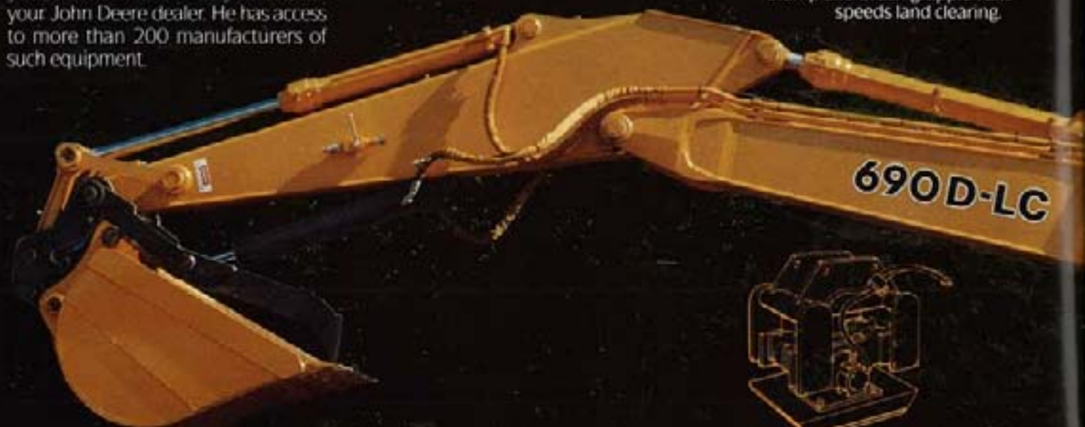
Vibratory compactor mounts in place of bucket, operates hydraulically.
