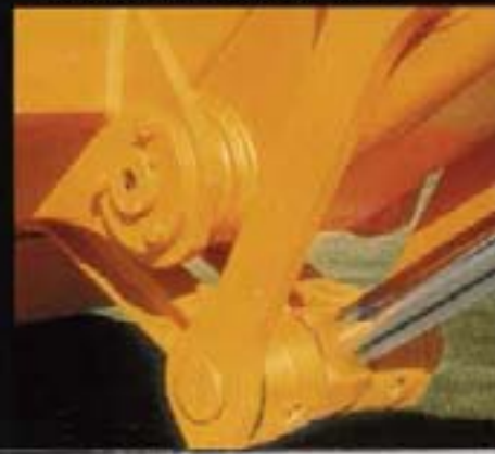
An adjustable bushing maintains the proper fit between the arm and bucket for better control, longer pin life.
