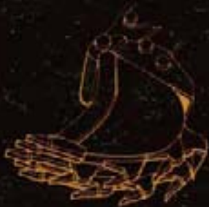
Ripper teeth on the back and the bottom of the bucket loosen frozen or hard ground or rock.
