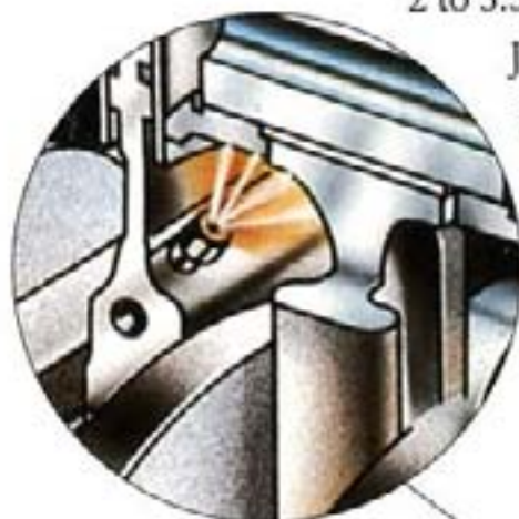
Jet-spray nozzles bathe the bottom sides of pistons with cooled oil for longer life.
