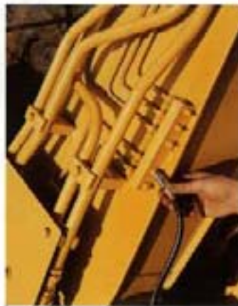
Remote lube bank lets you easily grease difficult to reach pivot points.
